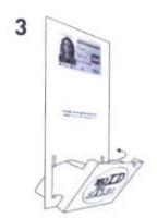
3. Push the side flaps (B) through the slots (A) on the printed back panel
